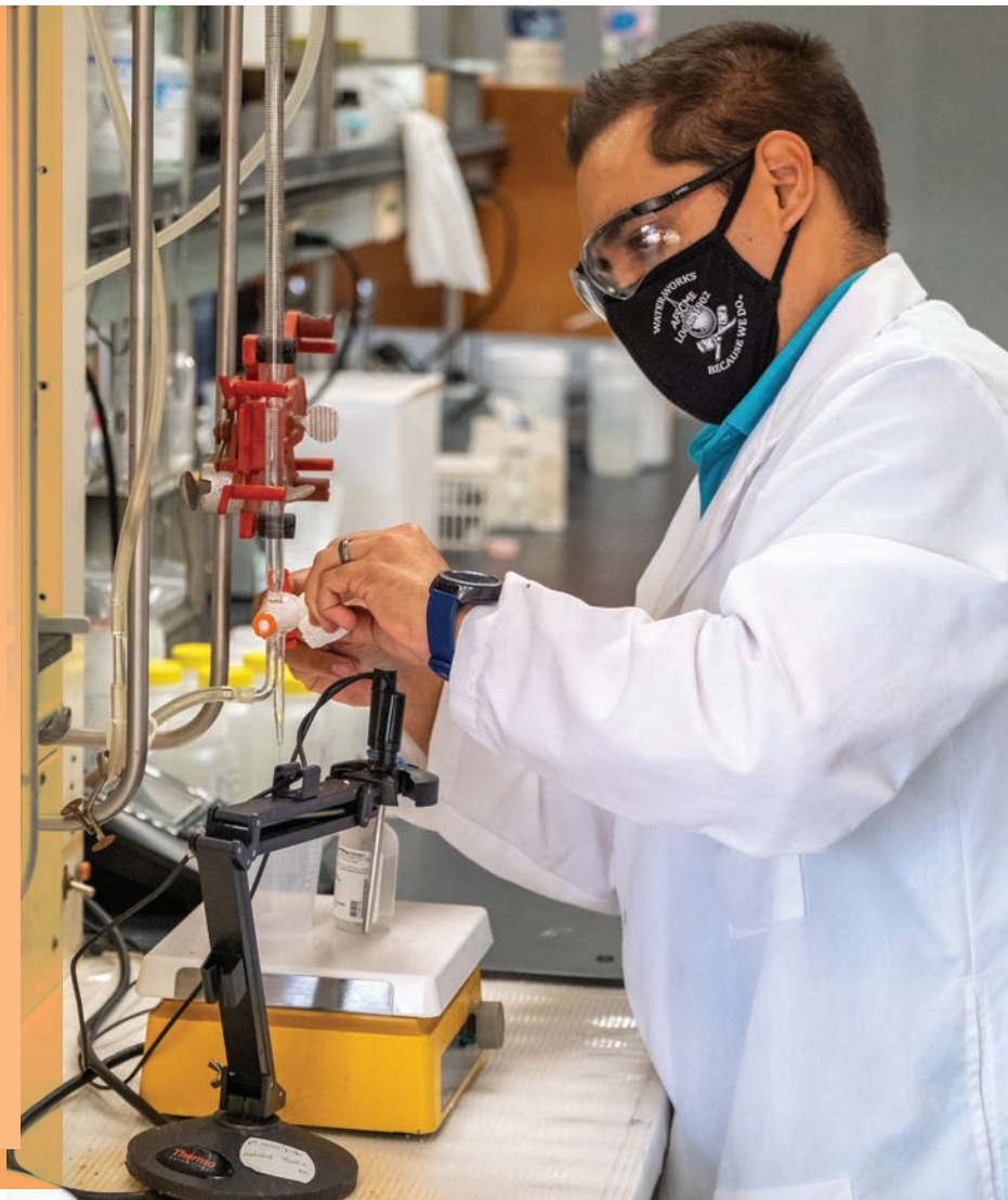
Associate Chemist Michael Olague titrating a water sample for alkalinity.
